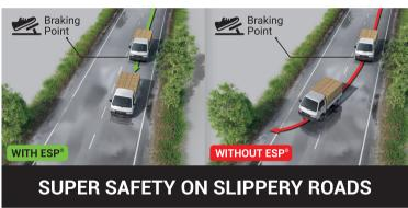
ESP® reduces skidding for better grip on wet surfaces, gravel, snow or loose soil.
